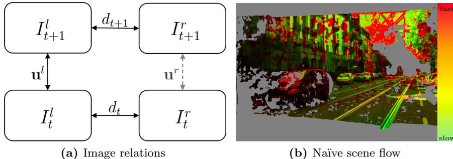
**Fig. 1:** (a) Relation of two stereo image pairs, (b) an exemplary result of scene flow reconstruction from stereo disparity and optical flow on KITTI dataset [4].
