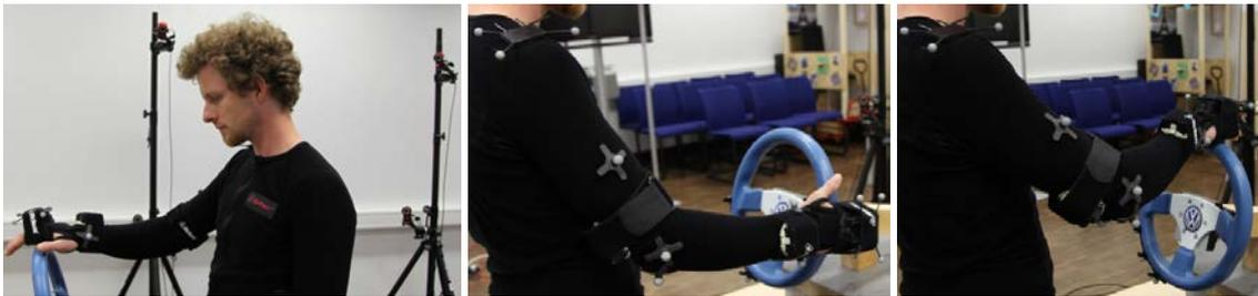
**Figure 1.** Measurement setup: stationary camera setup, attached markers and IMUs and start (middle) and end position (right) of the steering motion used in the experiments.
