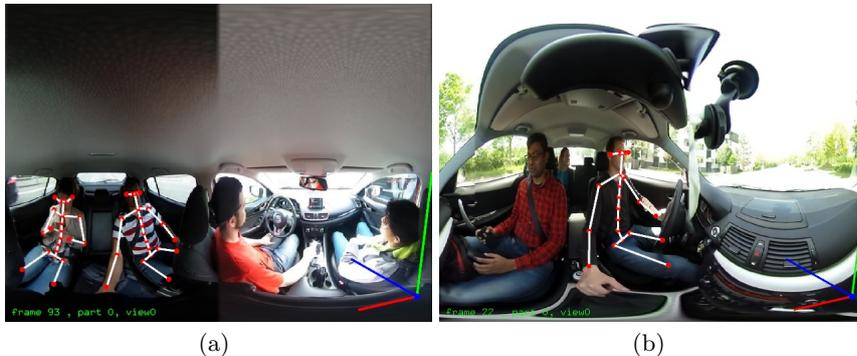
**Fig. 2.** 3D pose tracking of passengers with the 3D skeleton superimposed for (a) passengers and (b) driver
