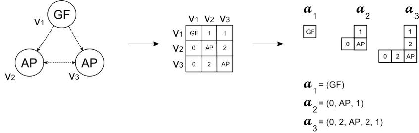
Fig. 1: The row-column representation of an adjacency matrix
