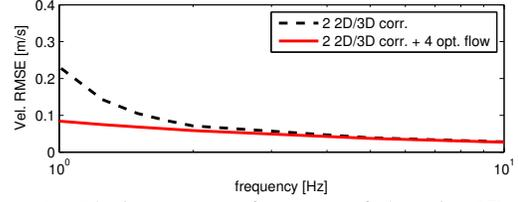
Figure 3: Velocity RMSE vs. frequency of observing 3D points.
