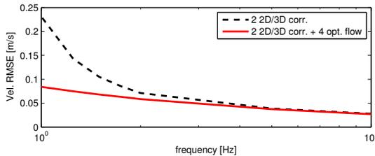
Figure 6: Root mean square velocity error vs. frequency of 2D/3D measurements from 100 Monte Carlo simulations. Two 3D anchor points are used. Note that these errors propagate time linearly into position.
