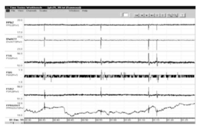
%FPG2 Intervalve gas fuel pressure input %FSR2 Gas fuel stroke reference from fuel splitter %FPRGOUT Gas ratio valve servo command %DWATT Generator load %FQG Gas fuel flow %FSG Fuel stroke reference
