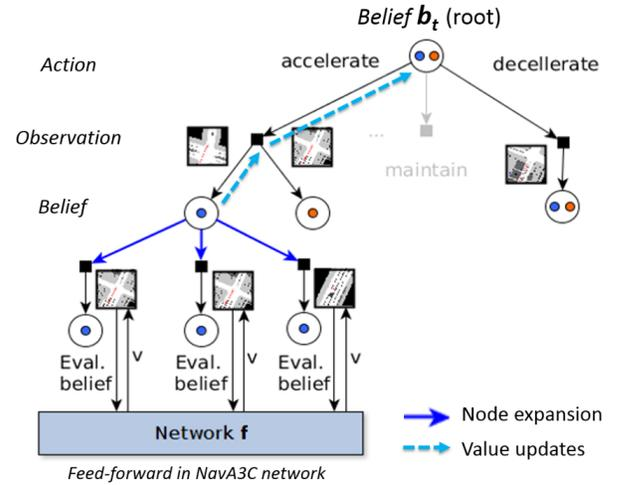
Fig. 5. Network-guided belief tree construction by IS-DESPOT at each simulation step  $t = 0..T$  of a traffic scene simulated in OpenDS
