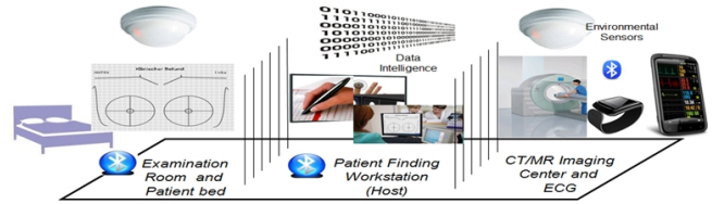
Figure 1. Architecture of the Medical CPS
